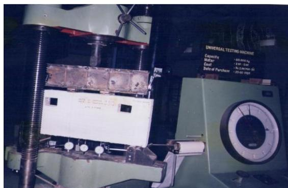
**Figure 2:** Test setup for deep beams
