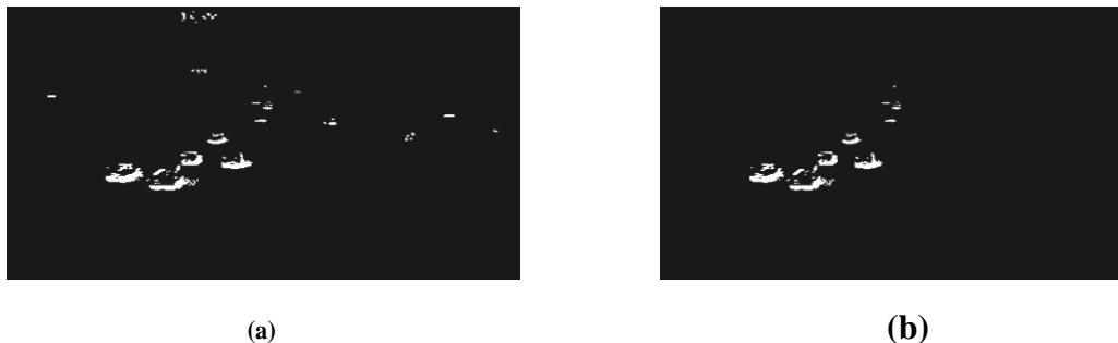
Fig 4: (a) Applying Binarization on the Image, (b) highlighting images and displaying the presence of vehicles in the targeted area
